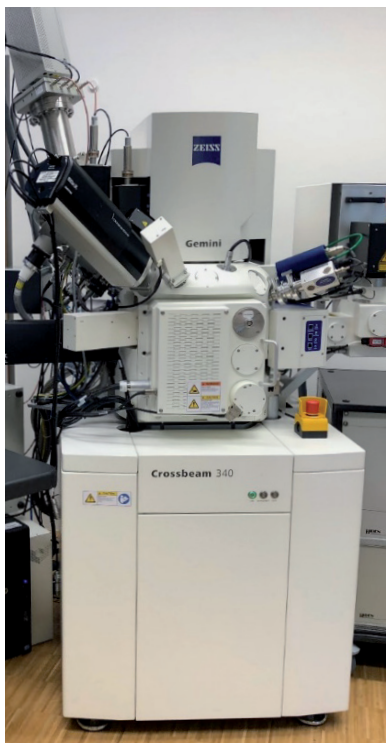
HIDEN EQS (top left) on Zeiss Crossbeam 340
