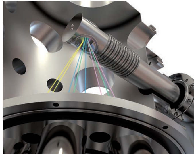
XBS Beam acceptance apertures
