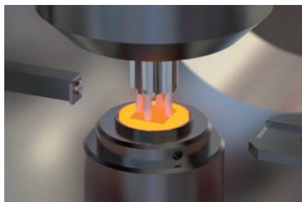
TPD Workstation with hot sample
