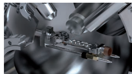
MAXIM SIMS/SNMS Spectrometer
