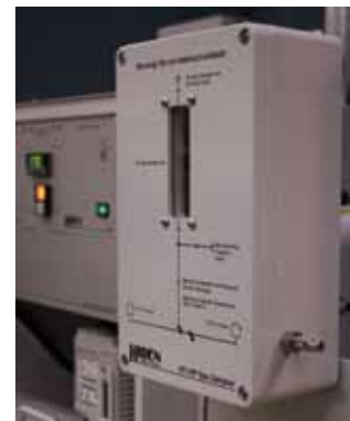
HT/HP inlet (up to 30 bar at 200°C)
